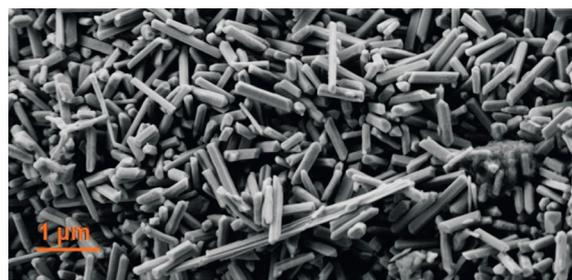
Fig. 2: Submicron  $\text{Bi}_3\text{Ni}$  by microwave-assisted polyol process.
