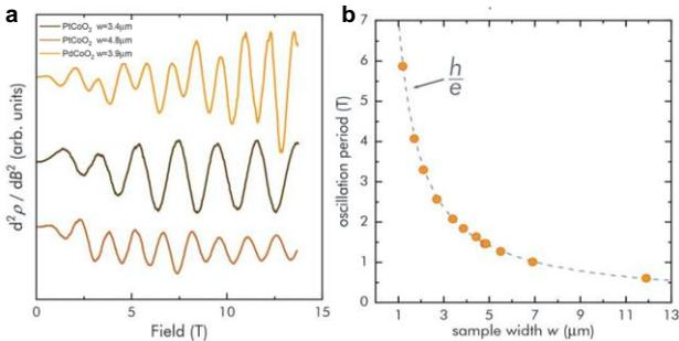
Fig. 3: (a) The second derivative of the resistivity highlights the oscillatory part of the magnetoresistance for three different delafossite samples. (b) The oscillation period is shown for different sample widths. The sample width dependence shows extraordinary agreement with the oscillation period expected for a single-particle magnetic flux quantum,  $h/e$ , per area enclosed by the sample width and the spacing between layers.
