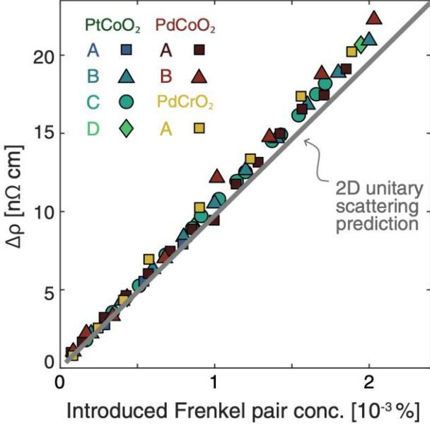
Fig. 1: Resistivity increment of four  $\text{PtCoO}_2$  samples, two  $\text{PdCoO}_2$  samples and a  $\text{PdCrO}_2$  sample as a function of introduced Frenkel pair concentration compared to the unitary scattering prediction.
