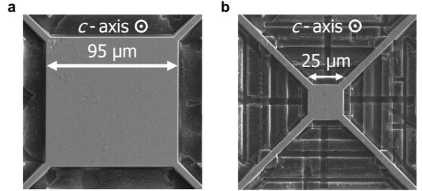
Fig. 2: Scanning electron microscope images, at the same scale, of a  $\text{PtCoO}_2$  square structured using a focused ion beam (FIB) with (a) side length  $95 \mu\text{m}$  and (b) with the edge size reduced to  $25 \mu\text{m}$  using the FIB.
